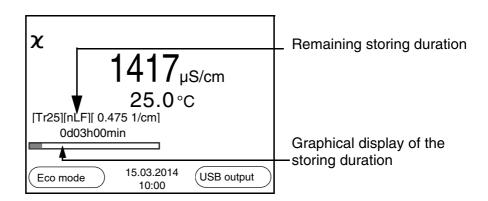
The active automatic data storing function can be recognized by the progress bar in the status line. The progress bar indicates the remaining storing duration.
